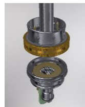
(3) Combustion chamber in TCA-08.
